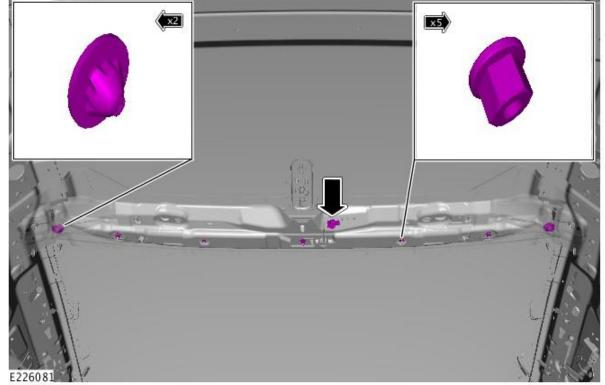
• Remove the 5 retaining nuts.
