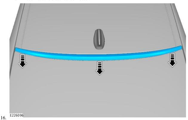
Remove the high mounted stop lamp.
