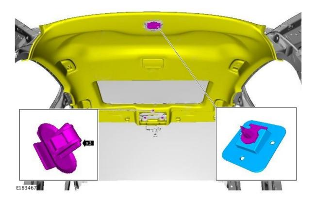
Release the headliner from the 3 front retaining clips and slide forwards to detach from the rear locating clip.
